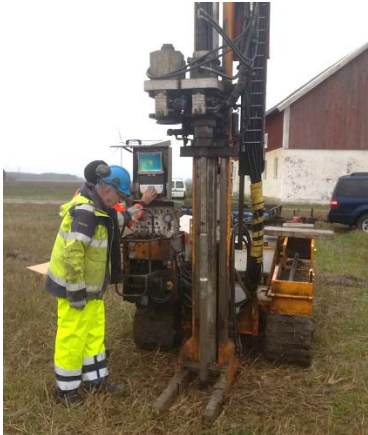
Figure 8. Taking soil sampling down to 0.8 m depth at Lanna.
